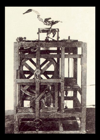
Vaucanson's Duck (1739) could flap its wings (with over 400 moving parts in each wing), eat, and (ostensibly) digest and defecate
